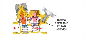
Alternately, the 1163xx series models incorporate a by-pass valve for thermal disinfection which is activated by a optional field mounted thermo-electric actuator, code 656 series, controlled by a automation system.
