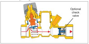
For systems using thermal disinfection for Legionella growth protection, the 1162xx series models incorporate a second thermostatic by-pass cartridge that activates at 160°F. A second flow path opens providing flow for the disinfection process which is independent of the primary balancing cartridge.
