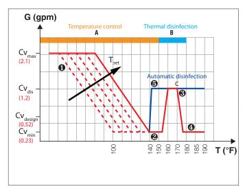
The graph shows the variation of the Cv value depending on the valve operating mode (A, B, C) and on the inlet temperature of the domestic hot water.
