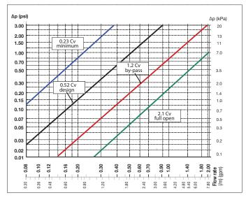
The "by-pass mode" curve in the chart above shows the head loss of the valve when it is in by-pass thermal disinfection mode for Legionella control.
